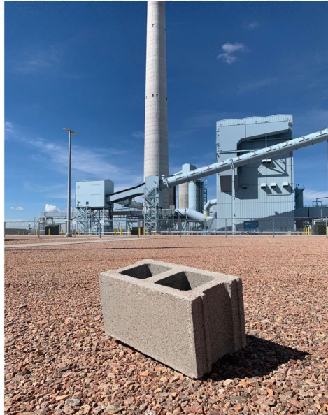
At the Integrated Test Center in Gillette, Wyoming, scientists from UCLA successfully injected carbon dioxide emissions from a coal-fired power plant into concrete, reducing the significant carbon footprint of concrete by up to 100 percent. The concrete blocks created using this technology cost no more to produce than traditional concrete and are now being used in the construction of several municipal projects across the State of Alabama.
